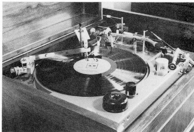
FIG. 3. Photograph of record-player cleaner in operation. (1) through (9), as in Fig. 2. (10) Stylus microscope (swivelling to pre-set position). (11) Arm stop positioned for microscope. (12) Lamp to illuminate stylus.
